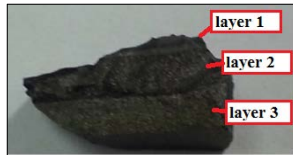
Fig. 15. FGM sample after ballistic impact.
