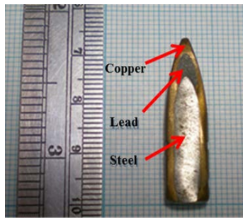
Fig. 2 Section of 0.30 armor-piercing bullet
